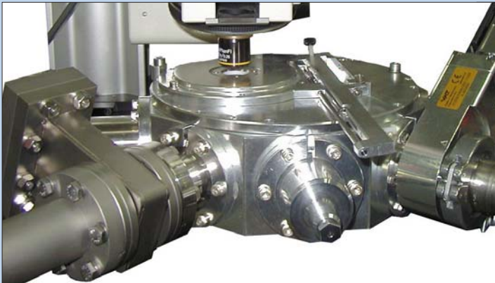
Cross-section of the vacuum chamber including cooling mechanism and AFM scan head
