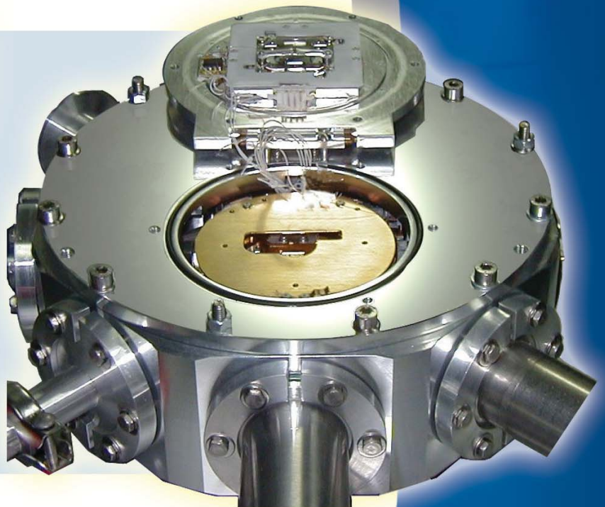
CryoView 2000™ vacuum chamber. The probe scanner is shown in the center of the open lid.
