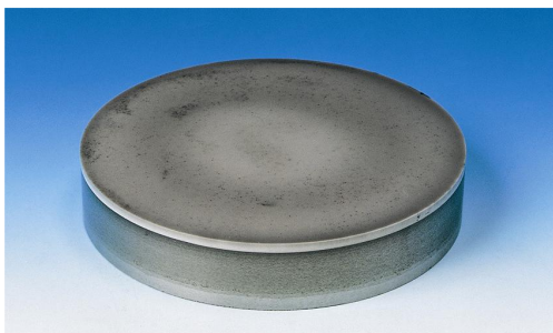
ZrO 2 /Stainless Steel FGM (100mm diameter)
