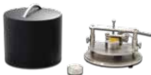
Room-Temperature sample holder with reference sample
